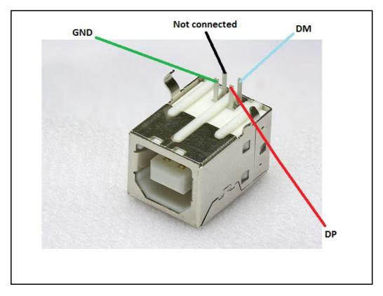
After soldering the three wires you can place a marker on each of them or use colored wires to be able to distinguish them. You can also use some gel to keep them tight on the USB connector. On the opposite side of the cables you might place 50mil (1.27mm) male connector following the order of the signals. Please also restrain from using wires longer than 20 cm since that might make the connection unreliable.
