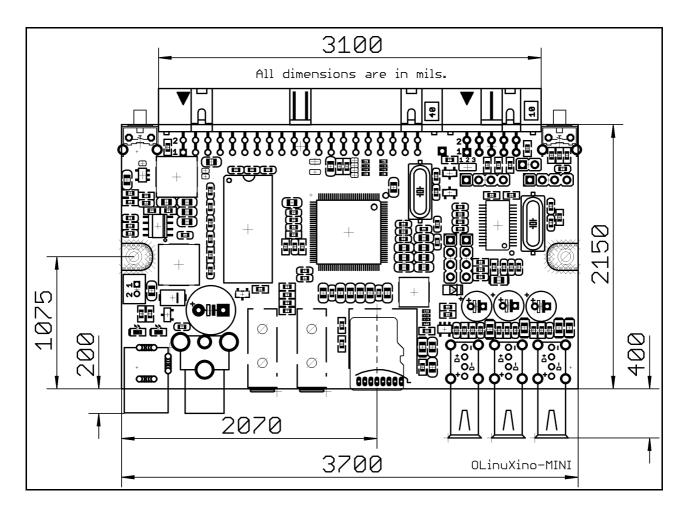
The three highest elements on the board in order from the tallest to the shortest are: capacitor C68 – 16.2mm (0.640") over the pcb; USB host connectors – 13.6mm (0.525"); composite connector – 12.0mm(0.464").
