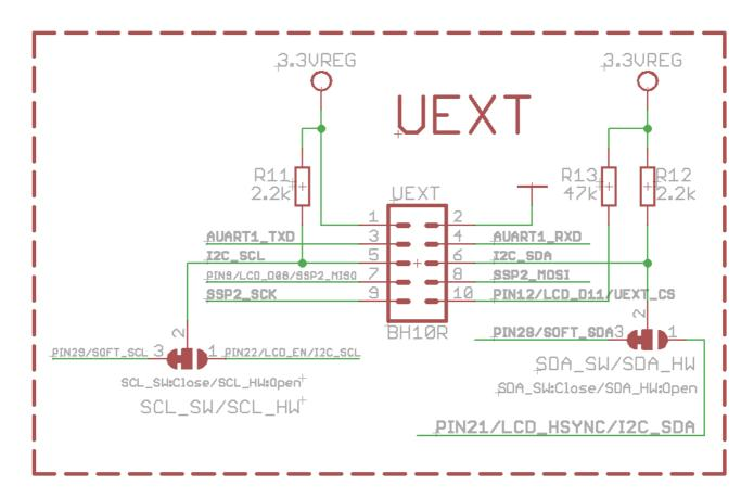
\*Note the two jumpers PIN29/SOFT\_CL – PIN22/LCD\_EN/I2C\_SCL, and PIN28/SOFT\_SDA3 – PIN21/LCD\_HSYNC/I2C\_SDA which by default are set to a software SPI. They can be used to set the whole UEXT to a hardware SPI.
