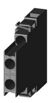
LATERAL AUX.SWITCH BLOCK,SIDE, 1NO+1NC, CURR.PATH: 1NC, 1NO, FOR MOTOR CONTACTORS, SZ S00, SCREW TERMINAL R: 21/22, 33/34 L: 41/42, 53/54
