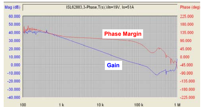
FIGURE 53. REFERENCE DESIGN LOOP GAIN T2(s) MEASUREMENT RESULT
