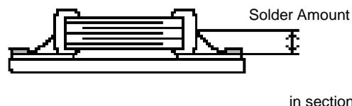
4-2. A Soldering iron with a tip of  $\phi 3\text{mm}$  or smaller should be used. It is also necessary to keep the soldering iron from touching the components during the re-work.
