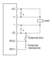
• When +S is not connected to the +terminal, and when -S is not connected to the -terminal, output voltage rises due to the sense amp open circuit. Output can then halt due to the overvoltage protection function. Also RV1 and RV2 should be left open if output voltage is not adjusted.
