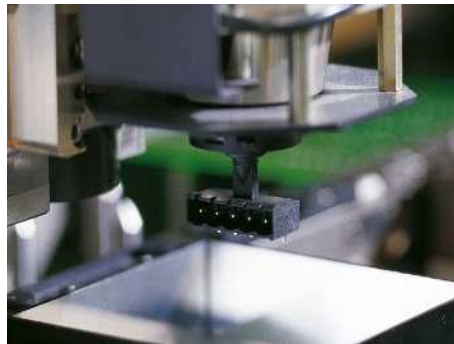
Camera recording for component measurement
