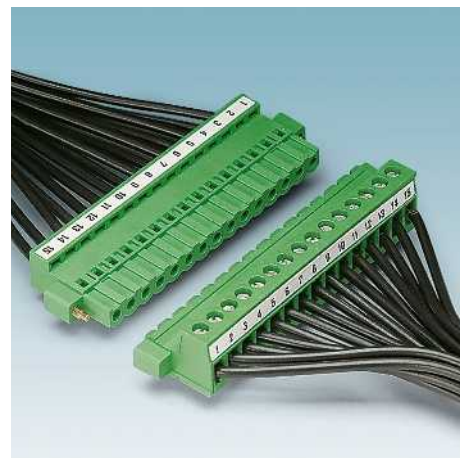
5. IC 2,5/... STGF with threaded flange for vibration-resistant free-hanging connection with MSTB plugs with screw flange.
