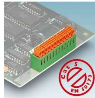
Displacement connection with 3.81 mm pitch, 0.5 mm² connection cross section IDC 0,3/...-3,81 Page 154
