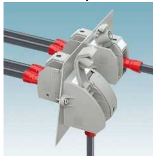
RW 8 series: bolt connection, up to 125 A, connection: vertical and horizontal RW 8...
