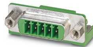
Shielded POWER SUBCON header for wall thicknesses of up to 4.5 mm, 4-40 UNC fastening thread, with leading medium PE contact
