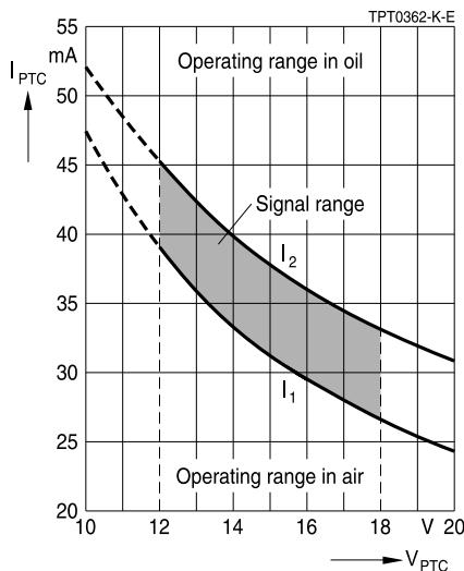
**Sensors****Point level sensor, glass-encapsulated, oil level sensing****E11****Reliability data**
