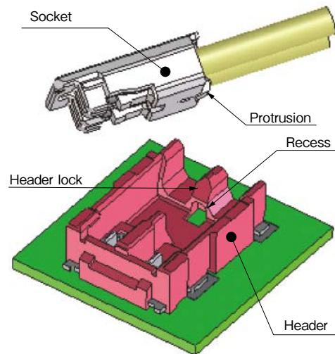
The protrusion on the bottom side of the socket fits into a corresponding recess on the header. This aligns the socket into the correct mating position.
