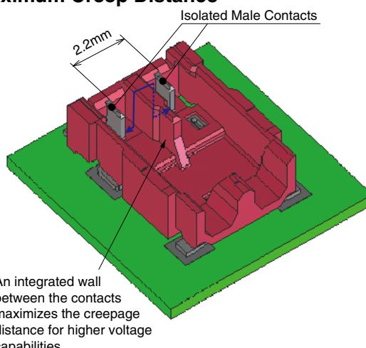
An integrated wall between the contacts maximizes the creepage distance for higher voltage capabilities.
