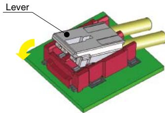
(3) Keep pressing down until a "click" feeling is sensed. The connector is now fully and properly mated.
