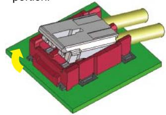
(3) Once the rear, or reinforced lock, is released the plug will come free from the header and complete the un-mating sequence.
