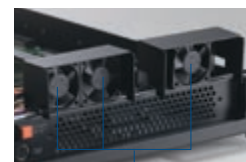
Three filtered 10-CFM cooling fans are on the front
