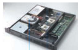
One internal 3.5" disk drive One rear 10-CFM cooling fan
