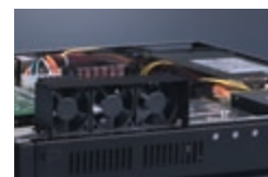
Three filtered 10-CFM cooling fans are on the front
