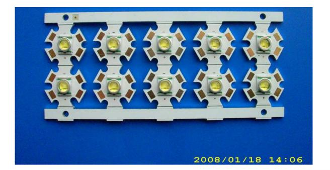
Star is nominal 20mm A/F. Centres for screw (e.g M3) mounting 17.5mm. MCPCB thickness is 2mm. Dimensions below in mm
