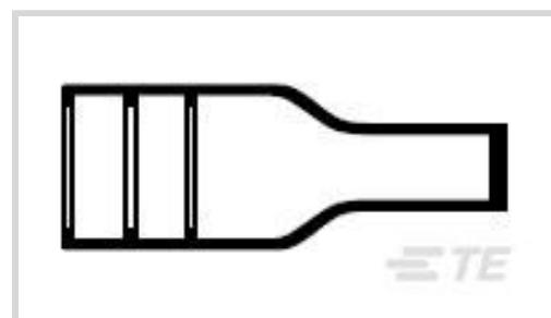
Body Orientation: **Straight**Molded Part Shape Code: **202**Lipped: **Yes**Material Code: **12**Material Systems Code: **200**
