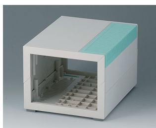
B2213205 MEDITEC E 160, without handle bar ABS (UL 94 HB) off-white RAL 9002 6.30"x7.87"x4.88" IP 40
