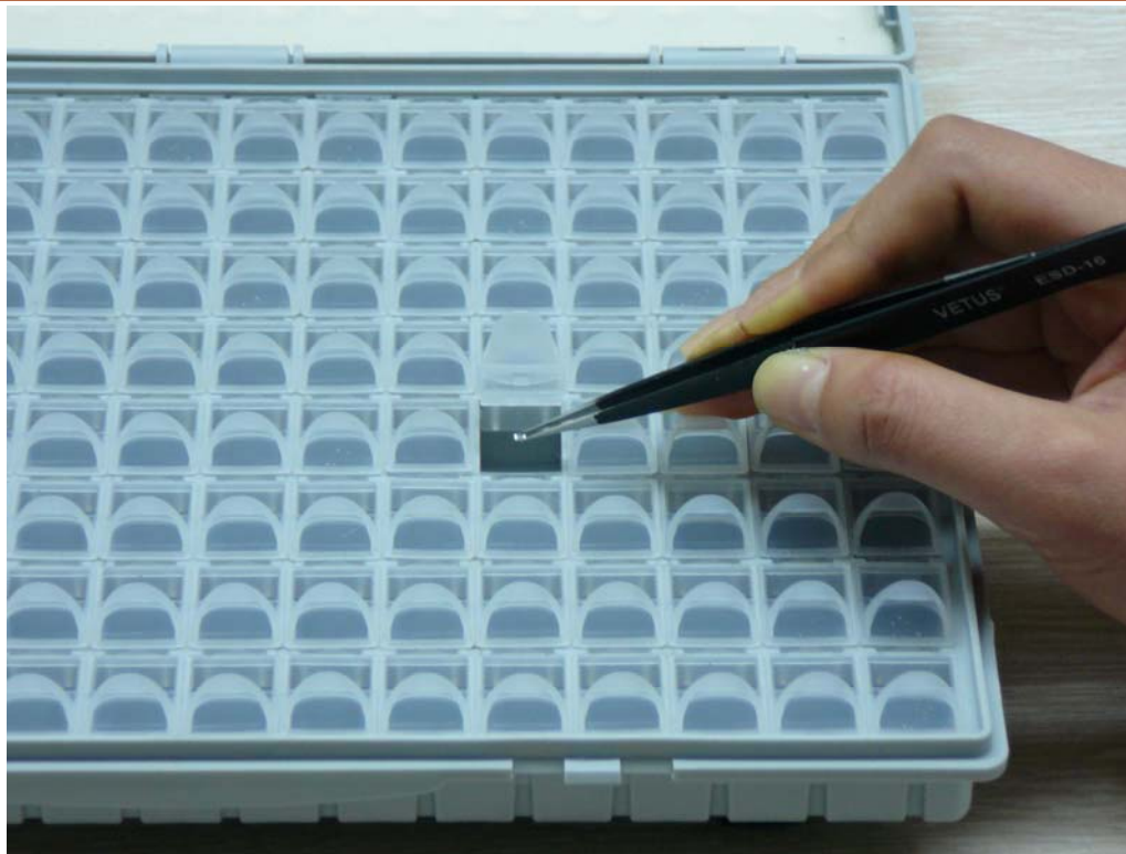
Figure 12. Storing or Obtaining an SMT Component
