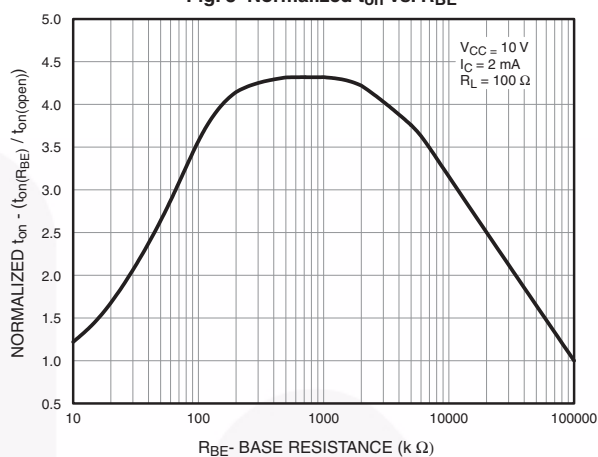
Fig. 8 Normalized t_{on} vs. R_{BE}
