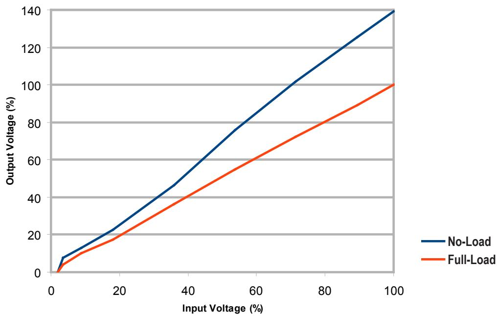
NOTE: The no-load curve may be as much as 200% x the full-load curve. Varies per model.
