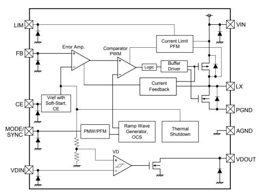
1A Driver Transistor Built-In Step-Down DC/DC Converters
