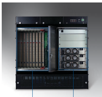
8-slot backplane with H.110 CT Bus
