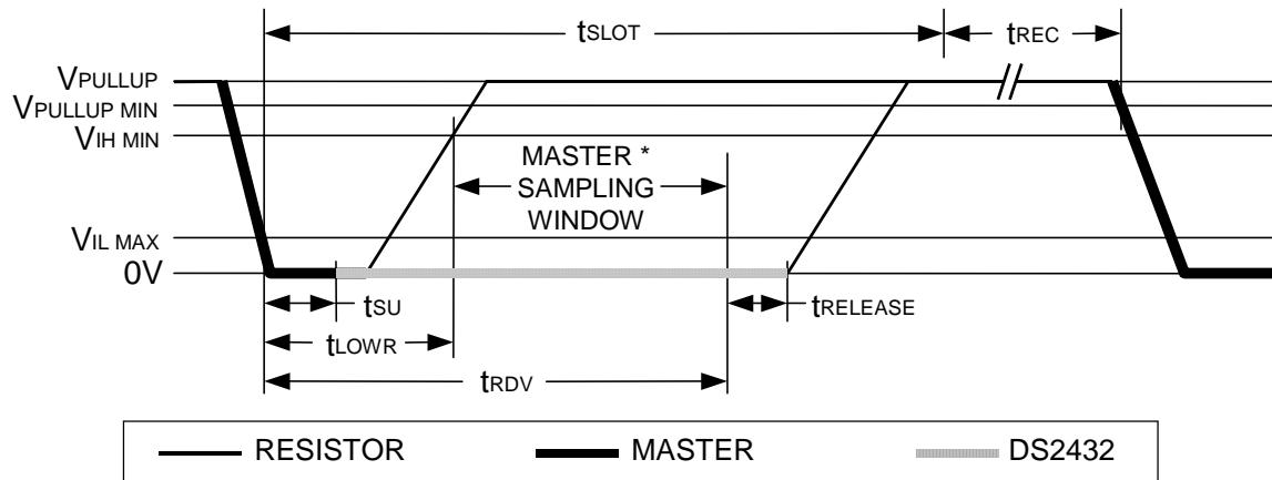
\*The optimal sampling point for the master is as close as possible to the end time of the  $t_{RDV}$  period without exceeding  $t_{RDV}$ . For the case of a Read-one time slot, this maximizes the amount of time for the pullup resistor to recover the line to a high level. For a Read-zero time slot it ensures that a read will occur before the fastest 1-Wire device releases the line ( $t_{RELEASE} = 0$ ).
