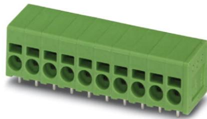
PC terminal block, Nominal current: 24 A, Nom. voltage: 400 V, Pitch: 5 mm, Number of positions: 11, Connection method: Spring-cage conn., Mounting: Soldering, Conductor/PCB connection direction: 0 °, Color: green
