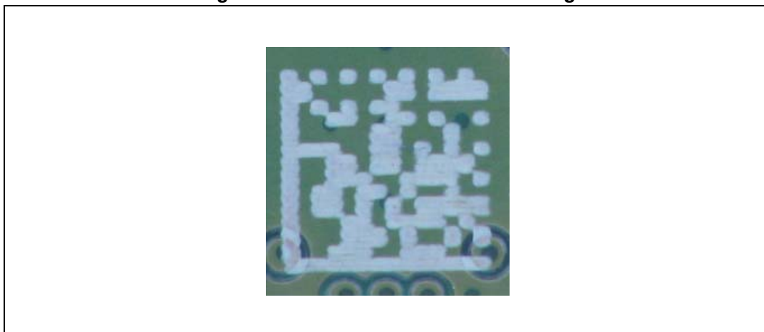
Figure 8. SPSGRF QR-code laser marking
