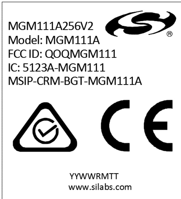
Figure 9.5. MGM111A Package Marking
