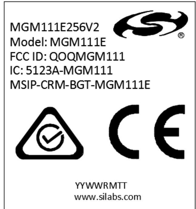
Figure 9.6. MGM111E Package Marking
