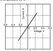
9. Input current vs. input voltage characteristics Ambient temperature: 25°C 77°F (Recommended input voltage: 5±0.5V)
