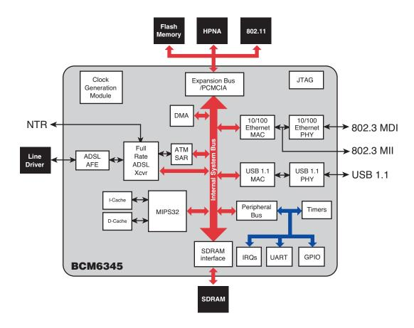
The **BCM6345** combines a G.992.1/G.992.2/T1.413 ADSL transceiver and AFE with a high-performance MIPS32<sup>™</sup> CPU, a 10/100 Ethernet interface, a USB 1.1 transceiver, a PCMCIA interface, and a generic and flexible expansion bus into a single chip.
