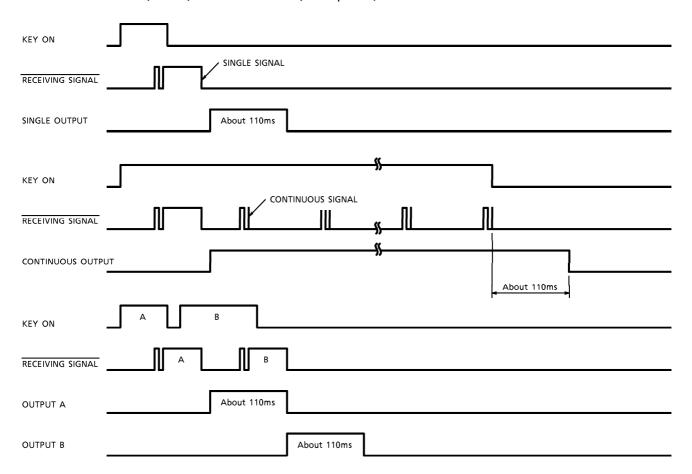
The hold pulse checks a system code of an initial single signal and a received signal and becomes "H" level only when data is valid.
