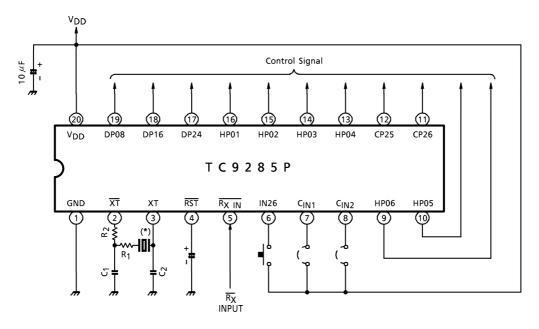
(\*) Ceramic oscillator CSB455E (Murata Seisakusyo)  $C_1 = C_2 = 100 \text{pF}$ ,  $R_2 = \text{unnecessary}$  In case of influenced by oscillation noise, add resistor  $R_1$  to  $10 \text{k}\Omega$  MAX. FCR455K3 (TDK)  $C_1 = C_2 = 220 \text{pF}$ ,  $R_2 = 4.7 \text{k}\Omega$ ,  $R_1 = \text{unnecessary}$  In case of influenced by oscillation noise, add resistor  $R_2$  to large (>4.7 k $\Omega$ ). or equivalent
