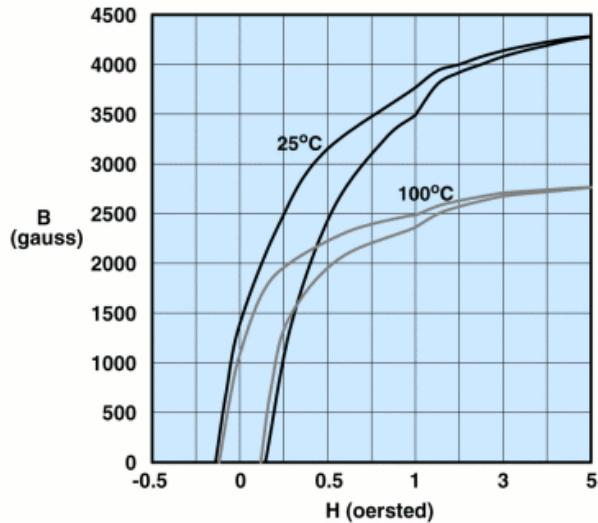
Measured on a 17/10/6mm toroid at 10kHz.
