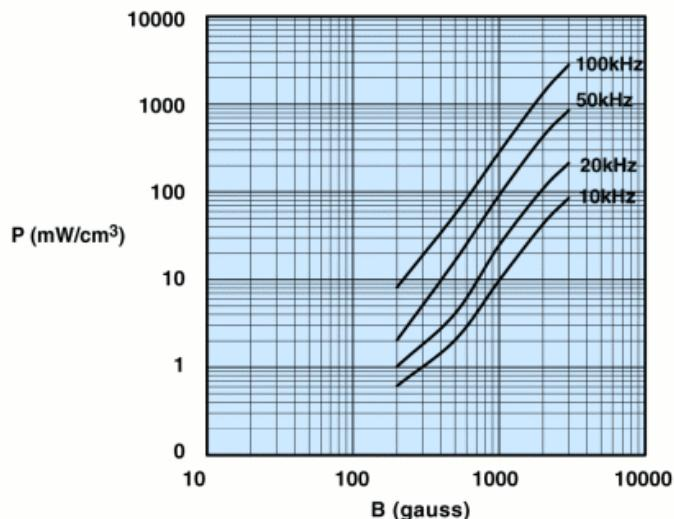
Measured on a 17/10/6mm toroid using the Clarke Hess 258 VAW at 100°C.
