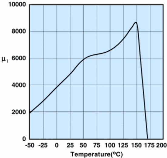
Measured on a 17/10/6mm toroid at 10kHz.
