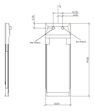
The SDC-EC15N is fully compliant with the PCI Express Card Type 1 mechanical standard. It can be inserted in any Express Card hardware interface and typically does not require any additional mounting hardware.
