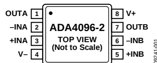
Figure 1. 8-Lead, MSOP (RM-8), ADA4096-2
