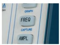
Quick and easy single-button capture function lets you acquire and store your signal directly from the oscilloscope's channels to the generator's internal memory. Not only can CH1 and CH2 signals be captured, but math functions applied to the channels can also be captured and stored.
