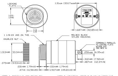
NOTE A: TERMINALS-032 BRASS TIN PLATED, TAPPED FOR #6-32 SCREW. TWO #6-32 NICKEL PLATED BRASS SCREWS INCLUBED. WILL ACCEPT 1/4' QUICK CONNECT. NOTE B: MOUNTING- REMOVE BLACK PLASTIC NUT
