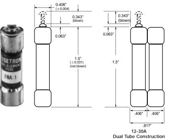
CATALOG SYMBOL: FNA (5AG) 1/10-10A DUAL-ELEMENT, TIME-DELAY 1/10 TO 30 AMPERES U.L. LISTED:
