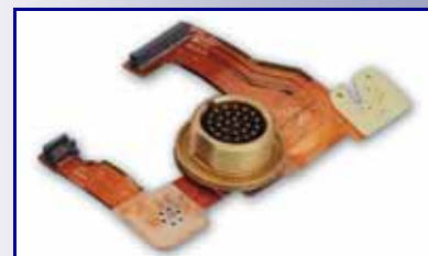
Flex Termination with MIL-C-26482 Special Connector
