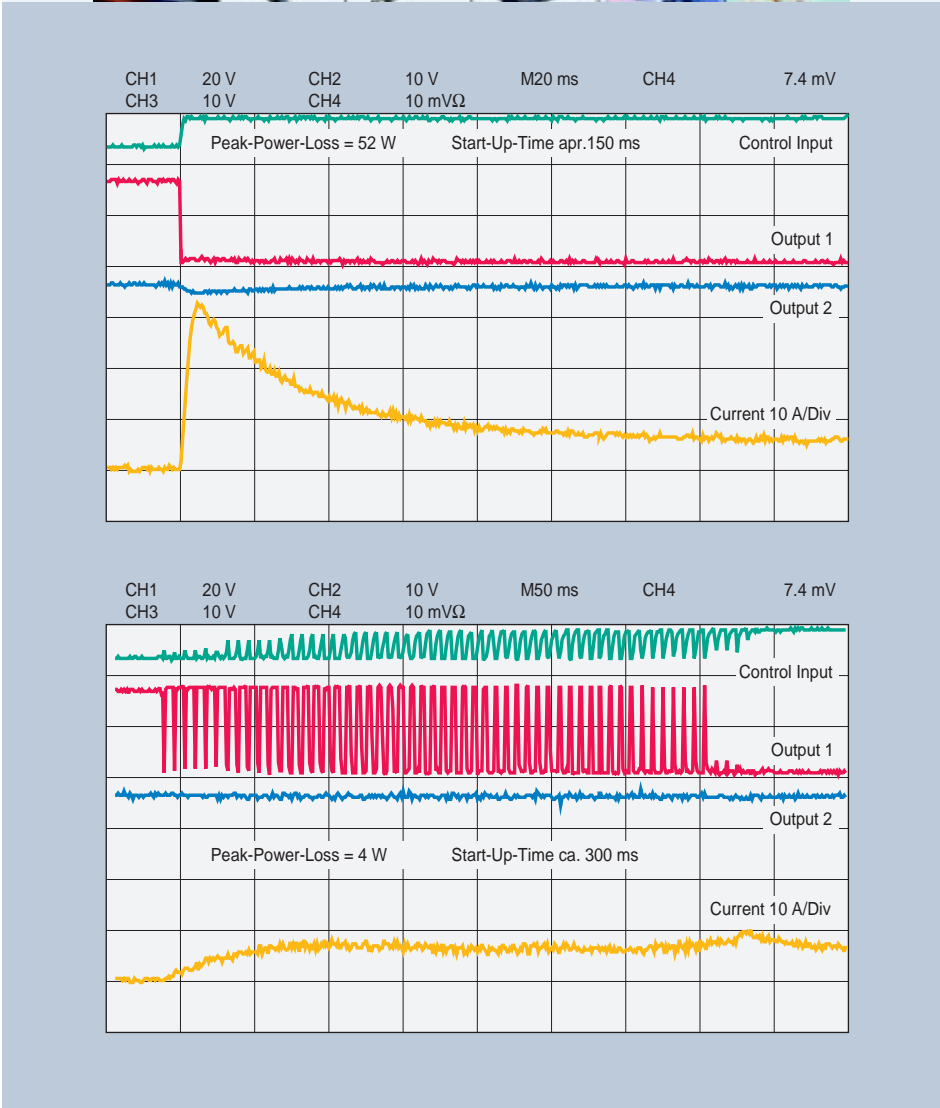
Figure 32 Start of a Power-Window Motor, V_s = 13\text{ V} . Upper: Hard Turn-on, Lower: Soft-Start
