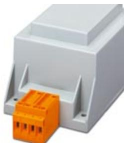
Molded transformer terminal block, Connection method: Screw connection, Length: 23.4 mm, Width: 12.4 mm, Height: 29.7 mm, Color: gray
