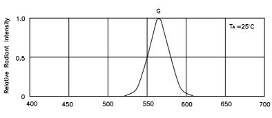
wavelength  $\lambda$  (nm) RELATIVE INTENSITY Vs. WAVELENGTH
