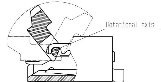
3. The actuator will not open more than 120°. Do not apply any force backward beyond this point. Otherwise, the actuator may come off or break.
