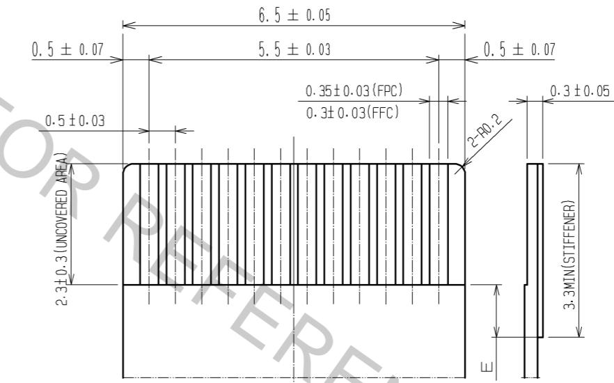
FOR FPC APPLICATION, STIFFENER MATERIAL IS POLYIMID, HEAT CURED ADHESIVE.
