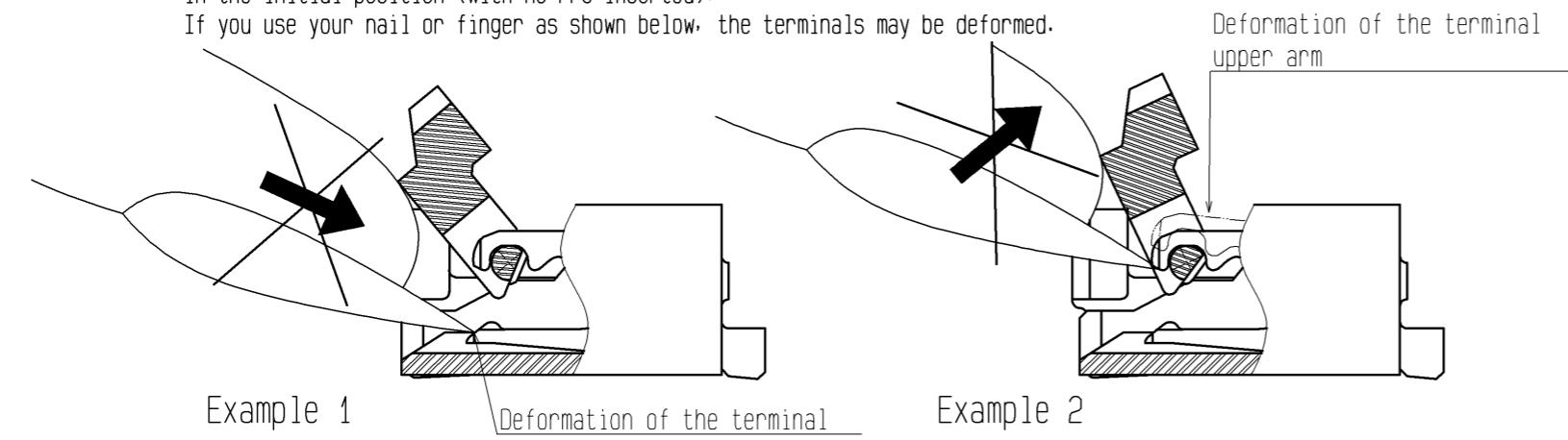
2. The actuator rotates around the rotational axis as shown below. Rotate the actuator.
