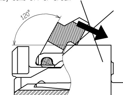
4. Move the actuator at approximately the center. Do not operate the edge of actuator. Otherwise, the actuator may come off or break.
