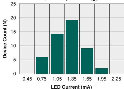
**Typical  $I_F$  for Switch Dropout
