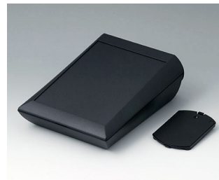
A0615119 COMTEC 150 H, Vers. II ABS (UL 94 HB) black RAL 9005 5.91"x7.87"x2.81" IP 40
