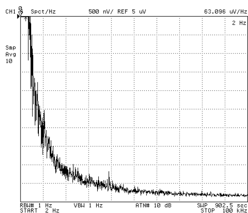
Input Voltage Noise vs. Frequency
