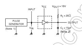
Note 1: Pulse Width 50 µs, Duty Cycle 10% Output Impedance 50  $\Omega$ ,  $t_f \le$  10 ns
