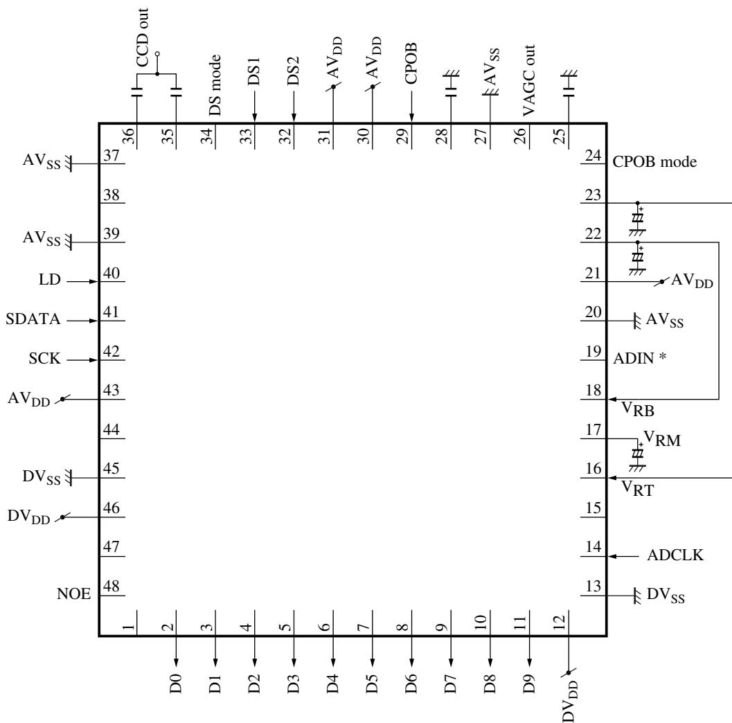
Note \*: When the AD amplifier is used, signals should be input to pin 19 through a capacitor. (Assumed chrominance signal may be input.)
