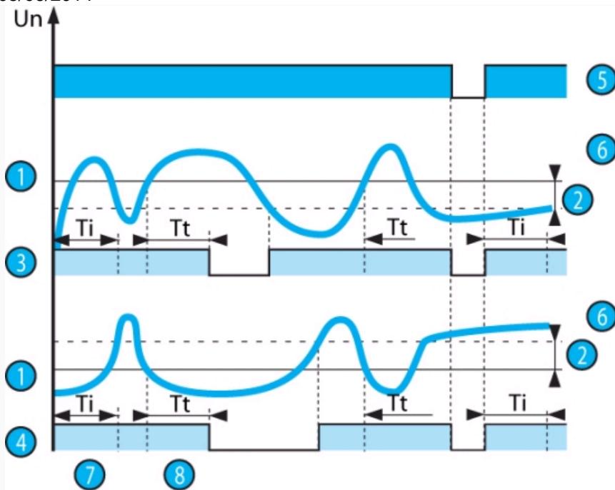
In overcurrent mode, if the controlled current exceeds the preset threshold for longer than the time set on the front face (0.1 to 3 s), the output relay opens and LED R is extinguished. During the time delay, this LED flashes.
