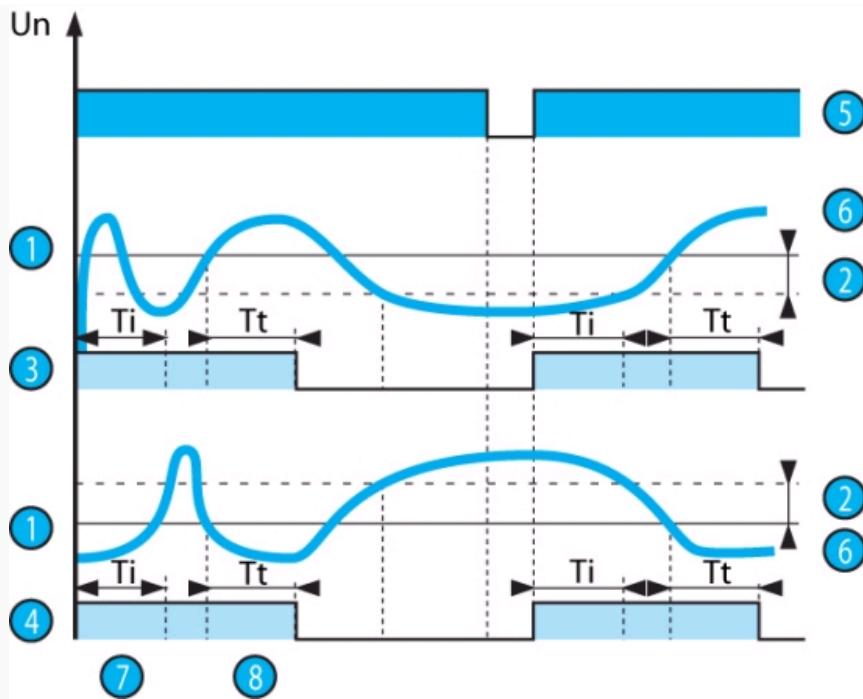
If "with memory" mode has been selected, the relay opens and stays in this position when threshold crossing is detected.
