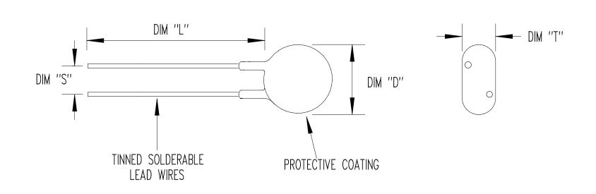
RESISTANCE @  $+25^{\circ}C = 10 \Omega \pm 20^{\circ}$
