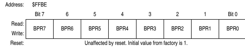
Write to this register is by a programming sequence to the FLASH memory.
