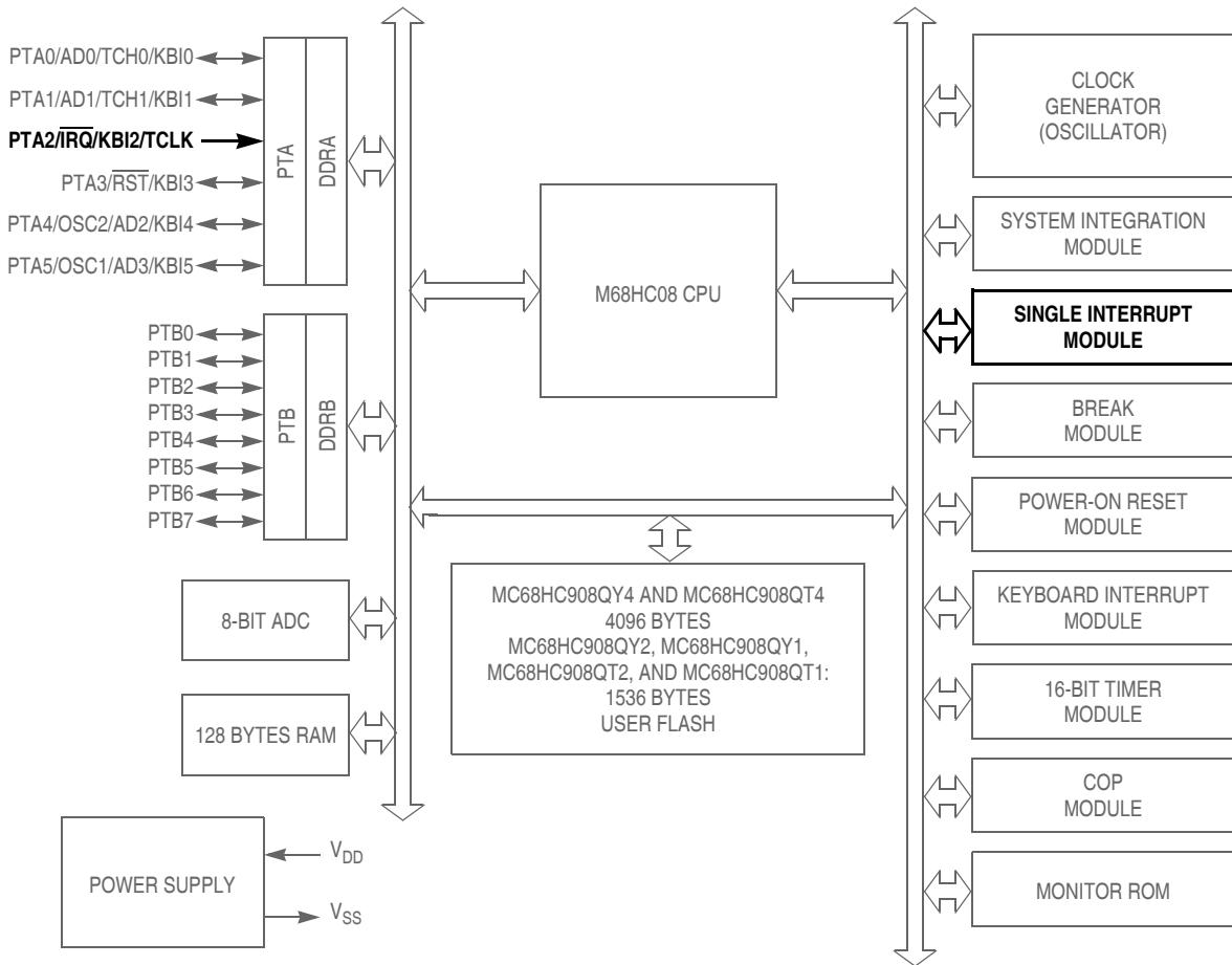
**RST,  $\overline{\text{IRQ}}$ :** Pins have internal (about 30K Ohms) pull up
