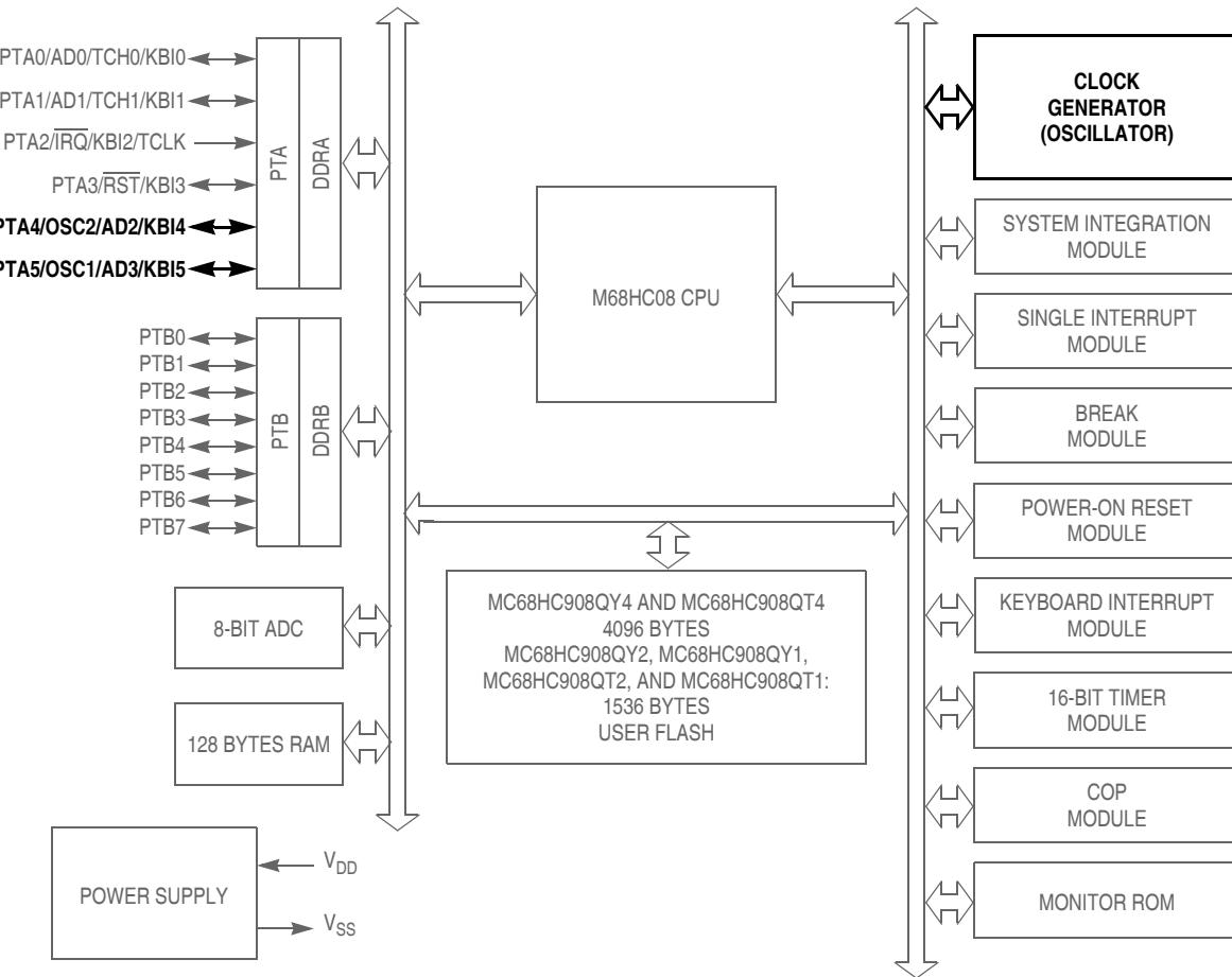
RST,  $\overline{IRQ}$ : Pins have internal (about 30K Ohms) pull up
