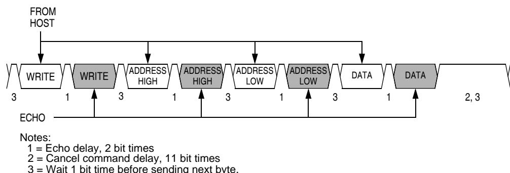
**Figure 15-16. Write Transaction**
