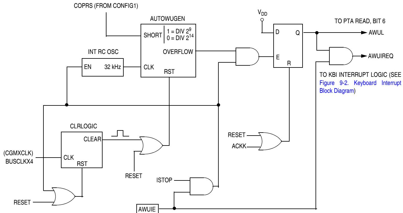
**Figure 4-1. Auto Wakeup Interrupt Request Generation Logic**
