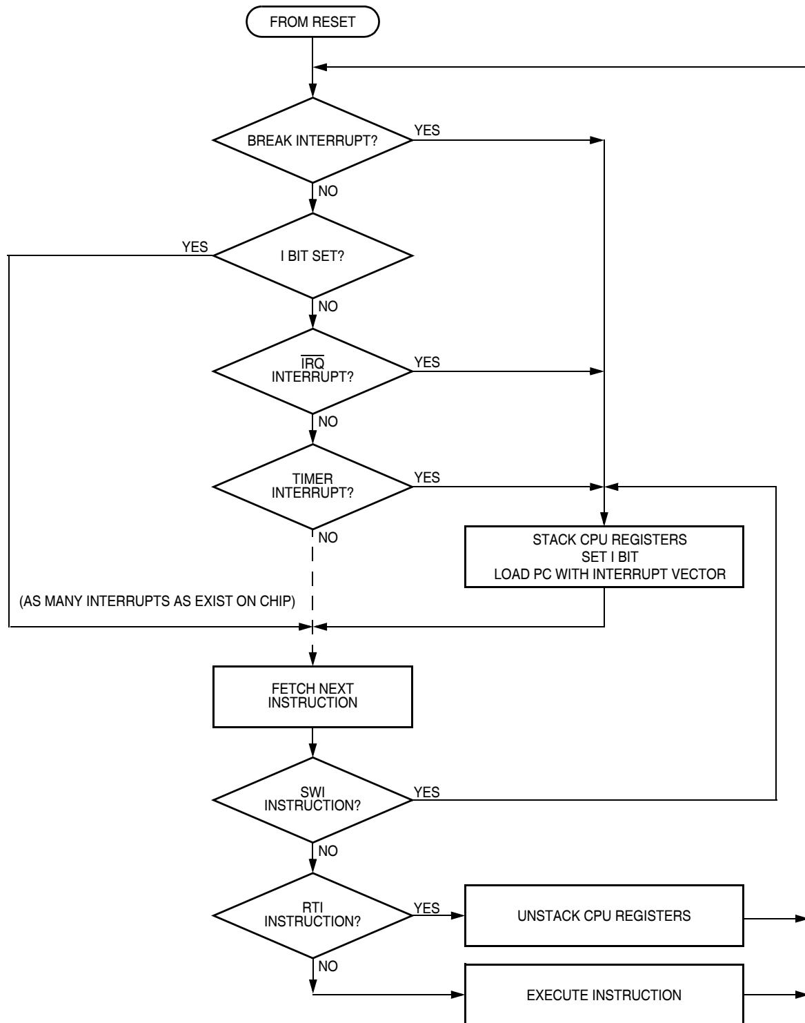
Figure 13-7. Interrupt Processing
