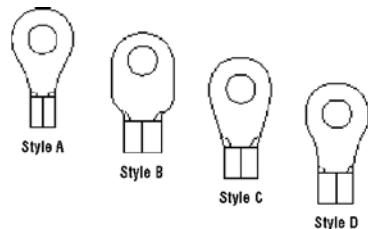
Terminal Body: Copper per ASTM B-152, tin plated per MIL-T-10727.
