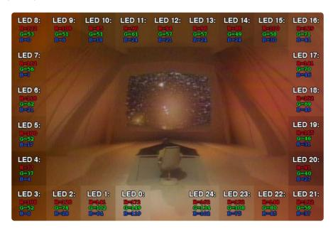
If you plan to arrange the LEDs similarly to our examples — 25 pixels in a ring, 1 pixel gap at the bottom, with the first pixel starting just left of the gap — then nothing more needs to be changed in the software. If using a different layout, you'll need to make adjustments in the code. You'll find extensive notes in the source code for making this (and other) changes.
