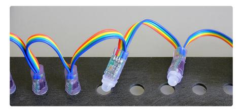
LED pixels can be press-fit into holes drilled through metal, wood or plastic. Holes 11 to 12 millimeters in diameter seem about right — experiment on a piece of scrap material first, find a size that gives a firm but not damaging grip.
