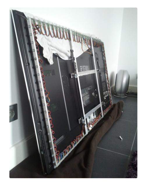
Forum user "Wackid" made this stunning 100 LED Adalight frame using aluminum Utrack with drilled holes carefully spaced around the perimeter. Extreeeeme!
