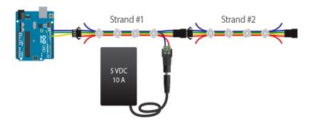
Wiring for 75, 100 or more LEDs is a little more complicated. You'll need some additional wire for distributing power, and a bit of soldering may be required.
