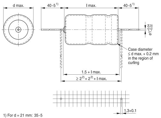
2) Minimum 2 mm bending distance per wire recommended
