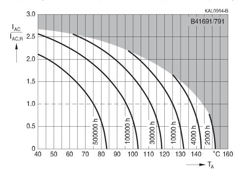
Useful life  $^{1)}$  depending on case temperature  $T_{\text{C}}$  under ripple current operating conditions at  $V_{\text{R}}$
