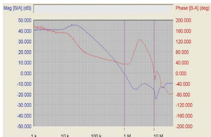
Figure 2 — Gain and Phase Bode Plot F_c = 810\text{KHz} , PM = 36 degree at 1A Source
