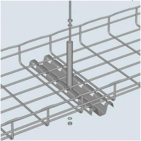
Only one threaded rod is needed to suspend tray.
