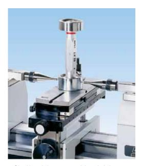
$\blacktriangle$  Checking of plug gages and threaded plug gages from dia. 1.18" to 10"/30 to 250mm using table (54-197-011), clamps (54-197-142), small  $\varnothing$  anvils (54-190-806) & thread wires (54-197-007)
