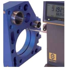
Internal measurements with ruby ball probe Ø3mm, 54-930-211
