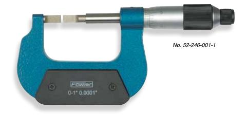
Use Fowler No. 52-246 Blade Micrometers to measure the outside diameter of workpieces which have narrow grooves, "T" slots and other dimensions blocked by shoulders or lands where standard type micrometers cannot be applied.
