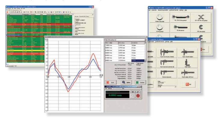
The QMSOFT (Quality Management SOFTware) system is a turn-key calibration package that enables the monitoring of a company's complete range of measuring and inspection equipment. To do this, QMSOFT uses a number of special modules which allow not only the management, but also the controlled measurement of gages.
