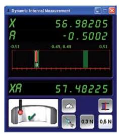
▲ Internal thread measuring display (Digital Display)
