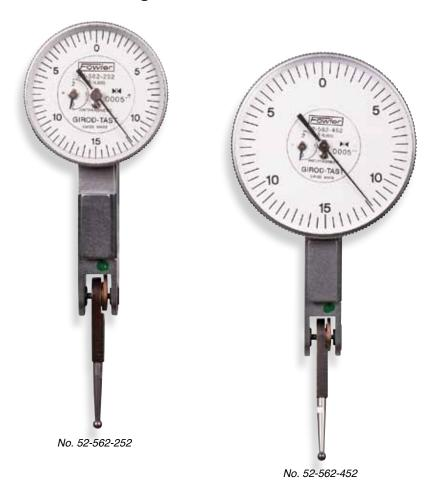
Fowler-Girod Test Indicators have long been regarded internationally as "the best." While retaining the Swiss quality and workmanship for which Girod has become famous, these indicators now offer a "double range" of .060". The new design also features a revolution counter hand to indicate the total number of revolutions of the main hand for fool-proof readings every time.
