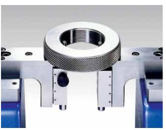
▲ Checking of threaded ring gages (low cost method) from minimum internal diameter of .70"(18mm), pitch from 0.25 to 5mm (4-80) thread per inch using floating cone holders (54-190-818), setting ring (54-190-804) and contact point cones (54-190-826)
