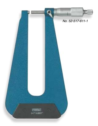
Fowler's "U"-frame Deep Throat Micrometers are available with depths of 6" and 12". Use Deep Throat Micrometers for taking accurate measurements of steel and plastic sheets and plates whenever a depth measurement of 2" to 12" is needed.
