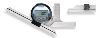
Fowler-Sylvac's Deluxe Electronic Protractor, featuring the patented Sylvac measuring system, provides an LCD readout in 1 minute of arc or 0.01 degrees of arc. A push-button selects the range according to application (1 x 360°, 2 x 180° or 4 x 90°) and changes the reading from arc minutes to decimal degrees. Additional push-buttons provide "reset" and "print" functions.
