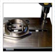
Internal measurement in 2 - points with auto-centering of the part on LVS 50  $\,$
