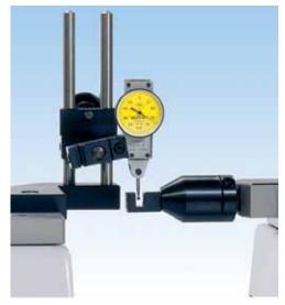
▲ Checking of lever (test) dial indicators using 54-197-115
