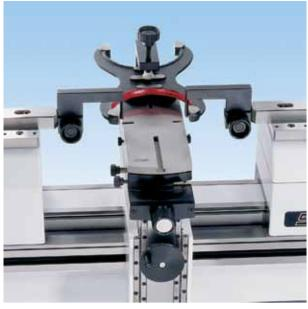
$\blacktriangle$  Checking of snap gages with range from .473 to 6"/12 to 150mm using table (54-197-011), snap gage holder (54-197-014) & L-probes (54-197-162)
