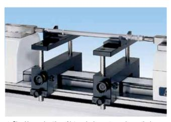
▲ Checking and setting of internal micrometers using vertical supports (54-196-107) & V-attachments (54-196-021)
