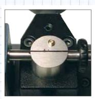
Table and anvils for internal measurement in 3 - points 1.3 - 2.5 mm
