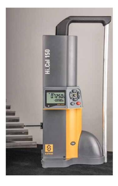
The Hi\_Cal XZ is a highly accurate 2-axis electronic height gage that was developed by Fowler and Sylvac for aircraft engine manufacturers. The Hi\_Cal XZ eliminates the need for multiple diameter gages at multiple depths.
