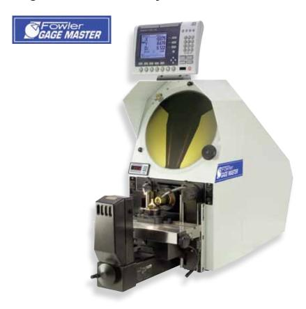
The Fowler bench mount profile projector with its 340mm screen combines high accuracy non-contact measurement and inspection with a large 175mm x 100mm measuring range.
