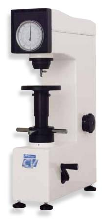
A high quality precision instrument that uses the Rockwell A, B, C and F scales for measuring hardness. A reasonably priced solution for those requiring precision and durability.
