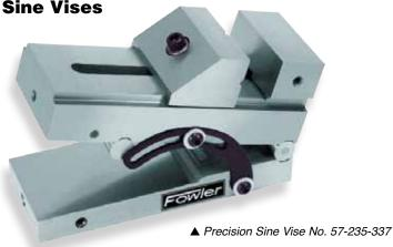
Fowler Sine Vises are precision toolmaker vises mounted to a precision hinged bottom plate. This provides a quick and accurate means of holding a workpiece at an angle for machining, drilling or grinding.
