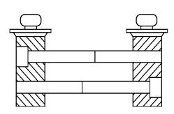
▲ 53-670-777 holding clamp set used for holding two large blocks together
