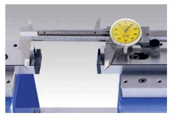
▲ Checking of calipers using 54-196-006
