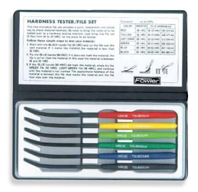
Fowler's Hardness Tester File Set is an inexpensive, easy-to-use method for determining material hardness by sliding the file across the object's surface. Six color coded files indicate hardness from 40 to 65 HRC. Conveniently packaged in a leather-like case with a velcro lined flap, the files are approximately .157" in diameter and 7" in length (4.30 x 175 mm).
