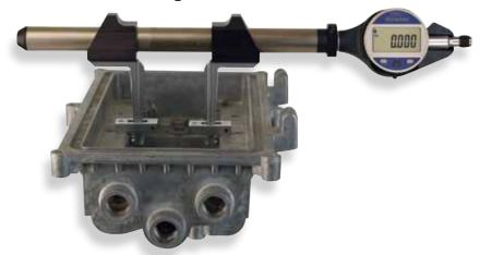
The Fowler/Bowers Universal Measuring Gage is ideal for the measurement of inside and outside diameters, threads, slots, recesses, grooves, tapers, etc. The large variety of accessories are easily and quickly interchanged, allowing measurements of virtually any type of workpiece.
