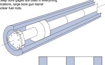
Can be fitted with spacers to allow segments to be measured throughout the depth of the bore.
