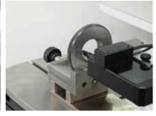
Checking of taper thread ring gages
