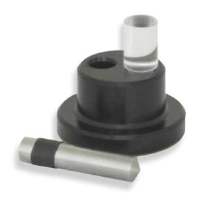
Place the acrylic lens in the holder to easily and accurately site in the area on the workpiece to be punched. Replace the lens with the center punch and quickly and accurately mark the workpiece.
