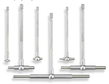
Another Fowler tool for easy and accurate measurements. Under spring tension, the plungers of the gage expand from the center to the size of the hole being measured and are then locked in place by a knurled knob. Final hole size is obtained by measuring over the contacts with a micrometer or vernier caliper.
