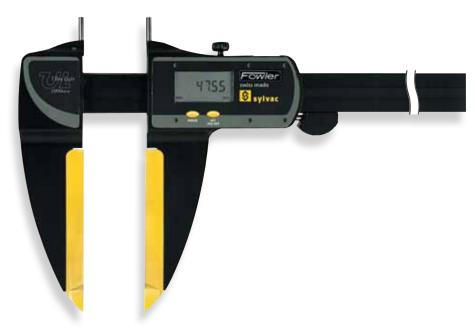
Fowler's Ultra-Lite Mark III Electronic Calipers offer many advantages over conventional calipers. Featuring a low weight that improves measuring results. Measuring pressure control for improved repeatability. For increased wear resistance, jaw faces are titanium-coated on hardened steel.
