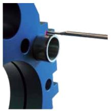
External diameter measurements with the standard probe 54-930-211
