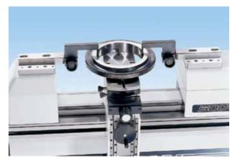
▲ Checking of ring gages from dia. .473"(12mm) to 10"(250mm) using table (54-197-011), clamps (54-197-142) & L-probes (54-197-162)
