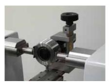
Checking of thread plug gages
