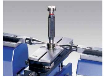
$\blacktriangle$  Setting of threaded plug gages from diameter 1.18" to 9.84" (30 to 250mm) using table (54-196-160), small Ø anvils (54-190-806) and thread wires (54-197-007)
