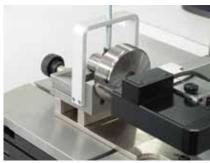
Checking of taper thread plug gages
