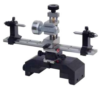
$\blacktriangle$  Checking of plugs 4" diameter (100mm), 11" length (280mm) part number 54-197-107
