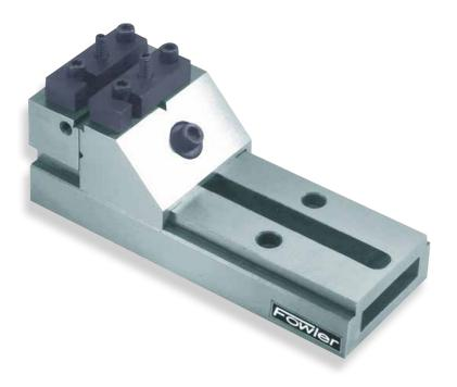
Fowler high-precision Toolmaker Vises have solid bodies of one-piece steel construction. Bodies and jaws carburized & hardened to RC58-62. All vises are ground flat, square and parallel within .0002" to .0003".
