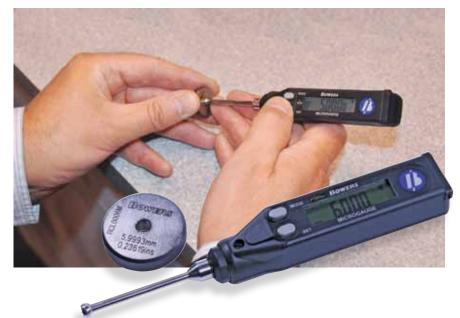
The new Fowler-Bowers MicroGage 2-point bore gaging system has been designed specifically for the measurement of small bores between 1.0 - 6.0 mm. The measuring heads are equipped with spherical, split-ball, hard-chromed contact points and are set in appropriate setting rings. The MicroGage system is available as individual instruments or as full sets. All setting rings are supplied as standard with UKAS certification.
