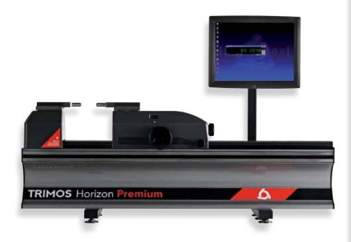
The Trimos Horizon Premium Length Measuring and Setting Instrument fulfills today's requirements of high accuracy quality control equipment. New superior engineering ensures the best measuring results by easy manipulation. The new Horizon Measuring System offers a wide range of accessories to meet numerous measuring and setting applications. Ideal for setting large ID/OD gages, bar gages and swing gages, etc.
