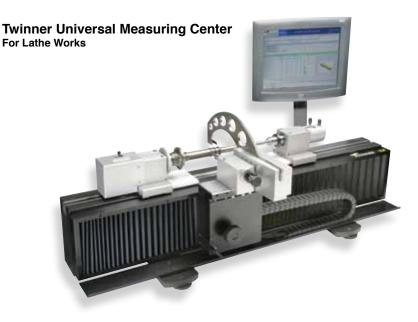
The Trimos Twinner is a multifunctional, flexible measuring center. Almost all parts that are manufactured with a lathe can be checked and documented. Precise measuring results of rotational symmetrical parts will be obtained in a short period of measuring time and without adaptation requirements.
