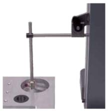
Internal groove measurements with accessories 54-199-508, 54-199-506 and 54-199-501
