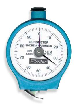
Fowler's Portable Durometers are just right for testing the hardness of flexible materials such as rubber and plastics. These gages conform to shore scales.
