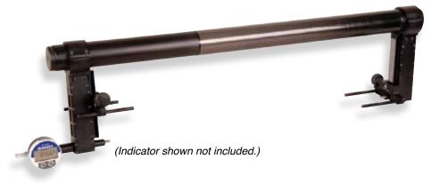
This light-weight gage allows one person to measure large diameter I.D. and O.D. measurements up to 80"(standard)
