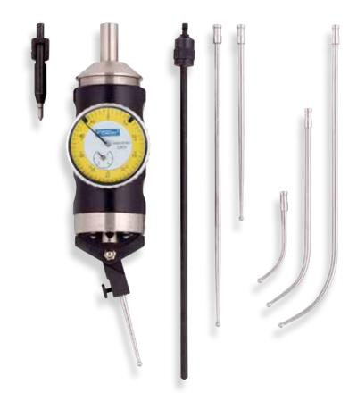
Use the 2D Coaxial Set for accurate component centering and positioning in most machining applications. The 2D Coaxial indicator can be used at any angle and the dial remains stationary during the rotation of the machine spindle.
