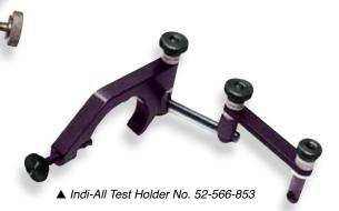
No. 52-566-853 Fowler's Indi-all indicator holder finds the center position without removing the tool from the machine. It mounts with a single set screw directly on the machine quill, bypassing the working tool. Use for milling machines, jigborers and Bridgeport mills (J-head).
