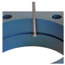
Internal groove measurements with accessories 54-199-508, 54-199-506 and 54-199-502
