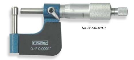
Fowler Rod-Anvil Tube Micrometers are positioned at a 90° angle in respect to the axis of the spindle, making it practical and convenient for measuring wall thickness of tubings and other workpieces with cylindrical walls.
