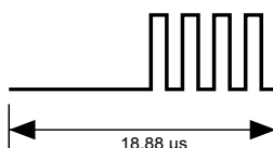
Figure 87. Logic 1, high data rate, fast commands
